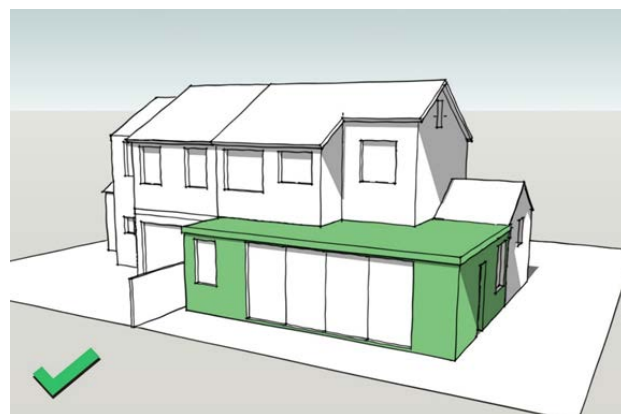
Figure 4: a property with more than one original rear wall. The example shows an extension that could be considered acceptable
