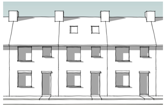
Figure 14: the correct positioning of roof-lights, in line with the existing windows at the first floor of the house
