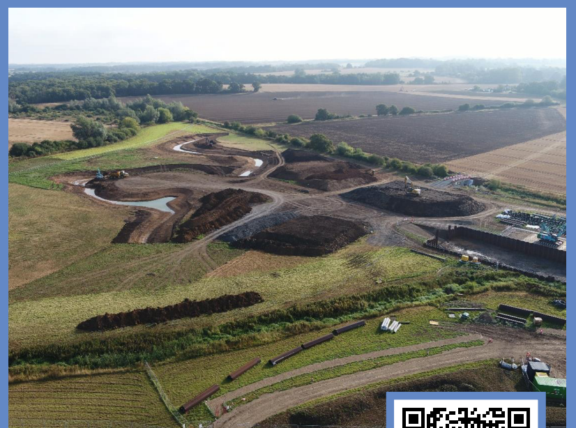
The site pictured from above, showing the river diversion works at the top and an excavated area for the new flow control structure on the right
