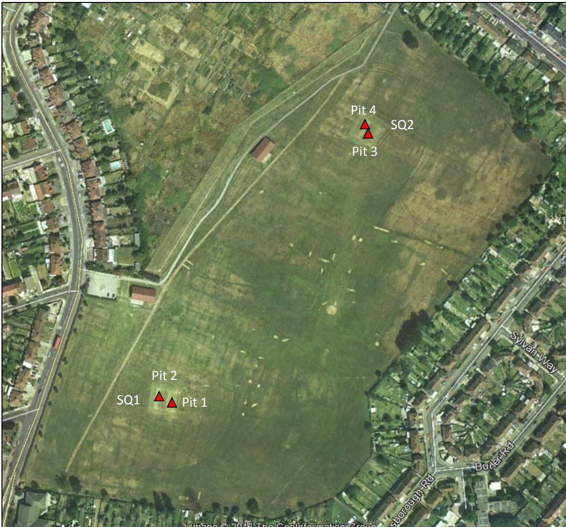
Figure 2. Goodmayes Park Extension and location of the two old cricket squares since abandoned and the shallow trial pits excavated in each square (image taken 2005).
