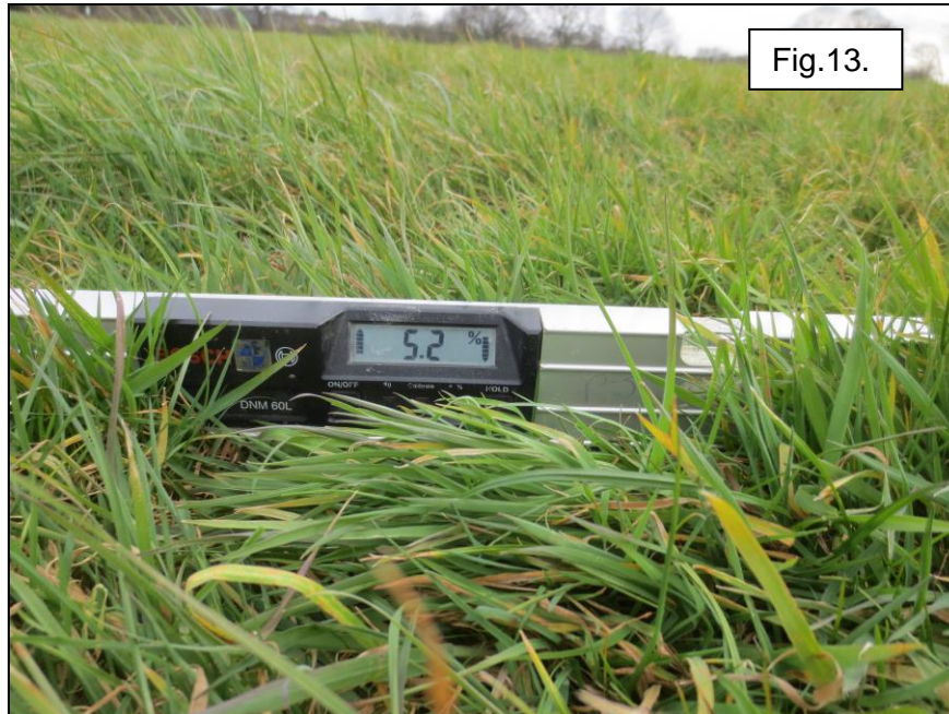
Steeper gradients in northern section falling towards river, ( 5% + ) meaning earthworks are required to alter gradients.
