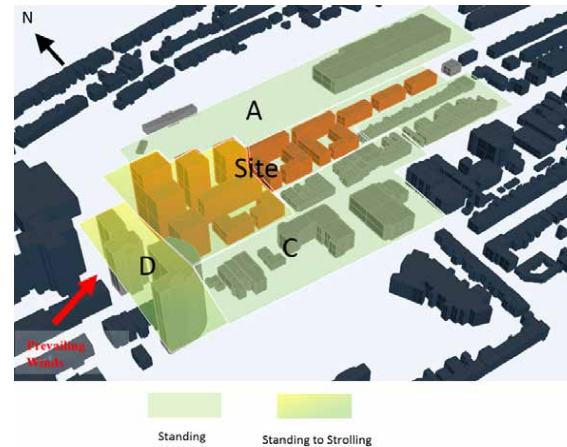
Figure 73 OS36 Wind microclimate assessment - high density scenario
