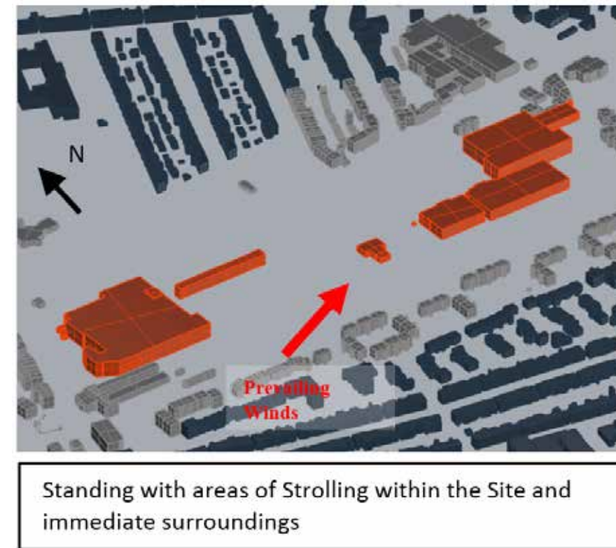
Figure 104 OS67&70 Wind microclimate assessment - high density scenario
