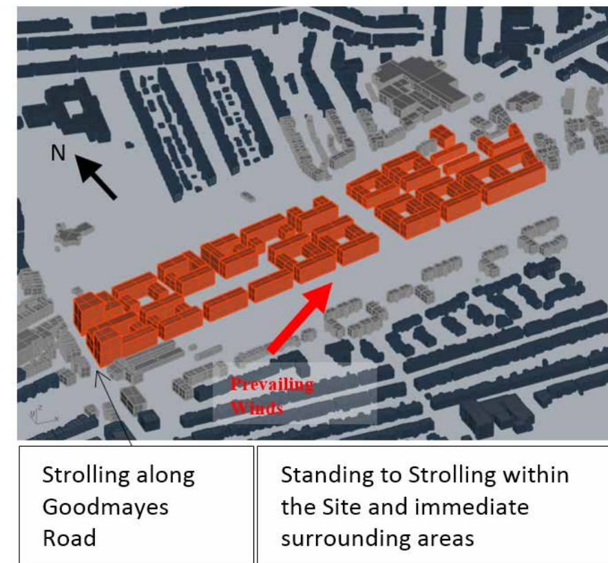
Figure 112 OS67&70 Wind microclimate assessment - medium density scenario
