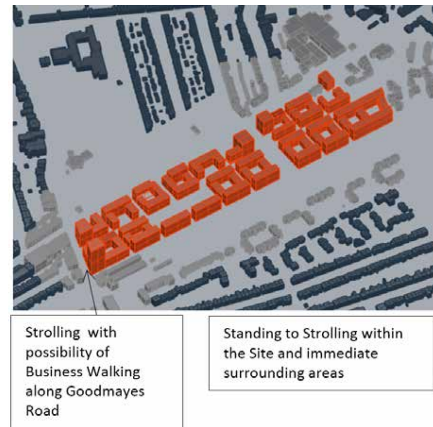
Figure 104 OS67&70 Wind microclimate assessment - high density scenario
