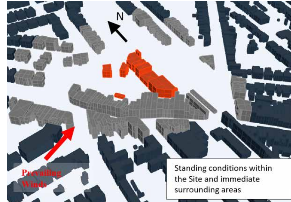
Figure 96 OS117 Wind microclimate assessment - medium density scenario
