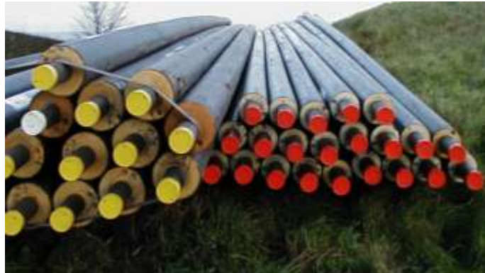
Figure 39: Rigid Steel pipes for District Heating (image courtesy of Ramboll)
