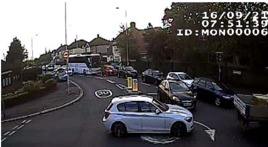
It should be noted that the second westbound lane is only 30 meters long, starts at the first lamp post on the right of the picture, vehicles turning right travel along the wrong side of Billet Road creating a pinch point for eastbound traffic.
